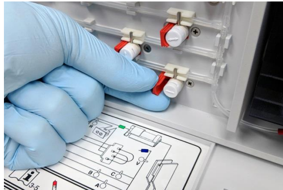
Figure 1-13 Removing red relief clamps
