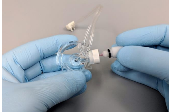
Figure 1-72 Remove Reference Electrode
