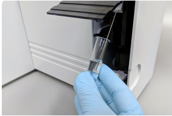
Figure 1-61 Sample probe in sample
