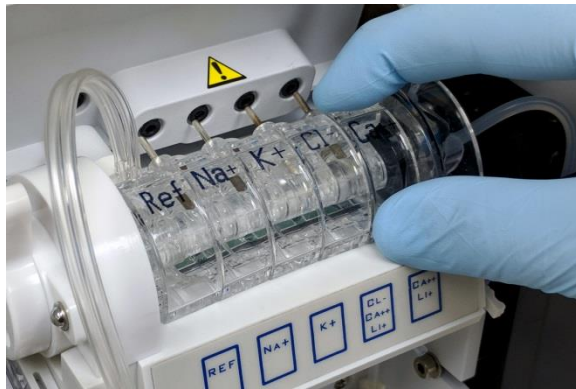
Figure 5-16 Electrode seated position
