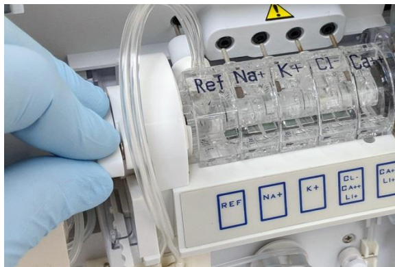
Figure 5-17 Rotate clamp down
