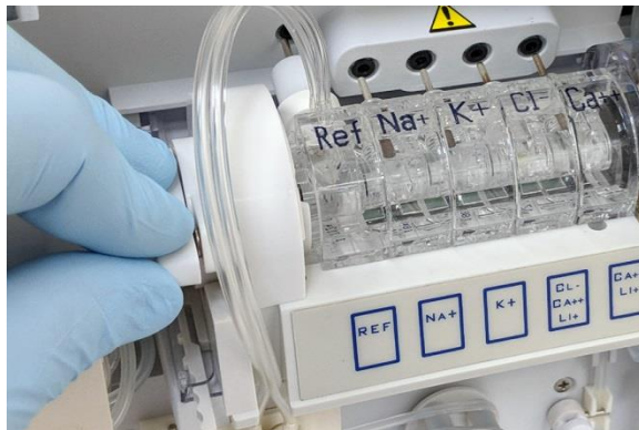
Figure 1-73 Reinstall housing with transport carrier
