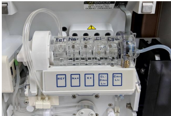
Figure 5-8 Push electrodes back into position.
