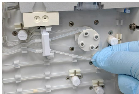
Figure 1-14 Pump windings on pump rollers
