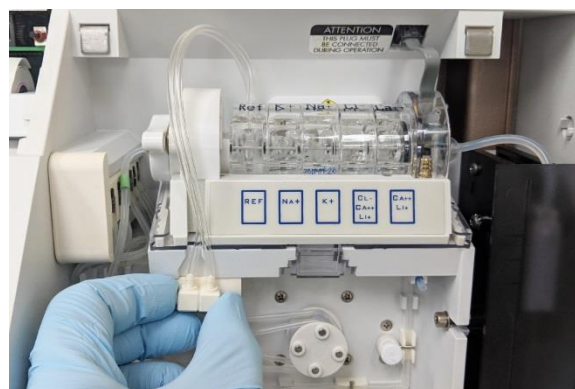
Figure 1-24 Plugging in reference connectors
