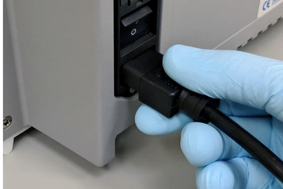
Figure 1-29 Connecting power cord to analyzer
