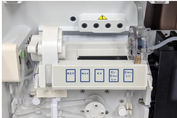
Figure 1-6 Electrode tray, locking mechanism closed
