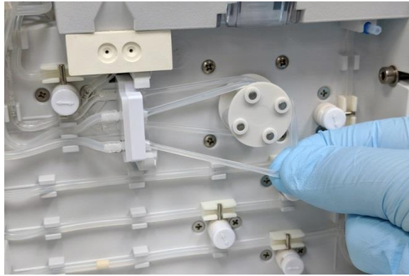
Figure 1-78 Remove pump tubing from pump roller
