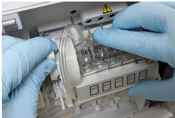
Figure 5-4 Move clamp to release tension
