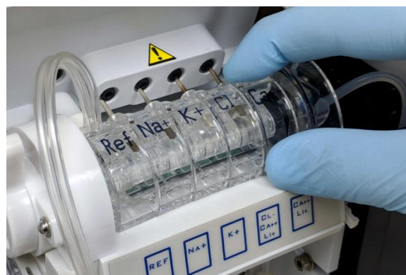
Figure 1-21 Electrodes in tray
