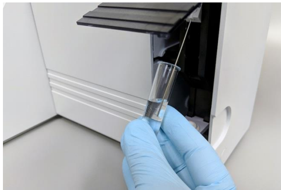
Figure 3-3 Sample probe in sample
