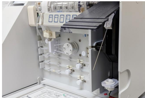
Figure 5-1 Open door for probe and port cleaning
