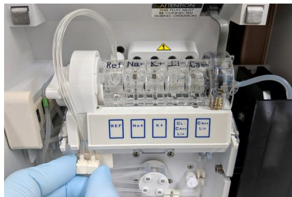
Figure 5-2 Unplug reference housing connector
