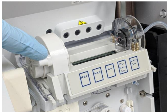
Figure 1-18 Electrode tray pulled forward (locked position)
