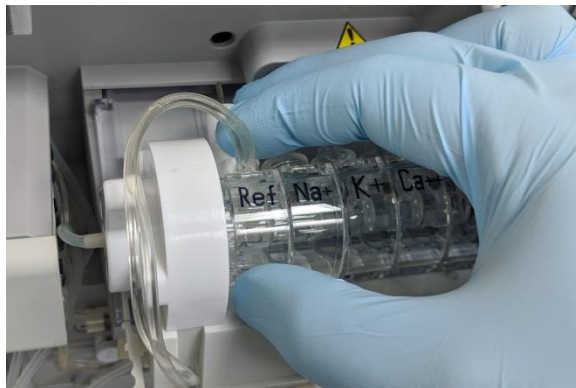
Figure 5-5 Remove reference housing and electrode
