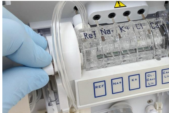
Figure 1-22 Move clamp down to locking position
