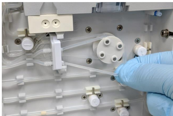
Figure 5-9 Un-wind pump tubing
