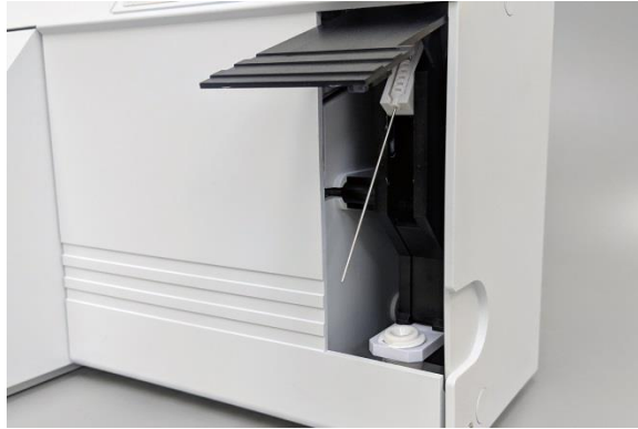
Figure 1-8 Opened door with Sample probe in
