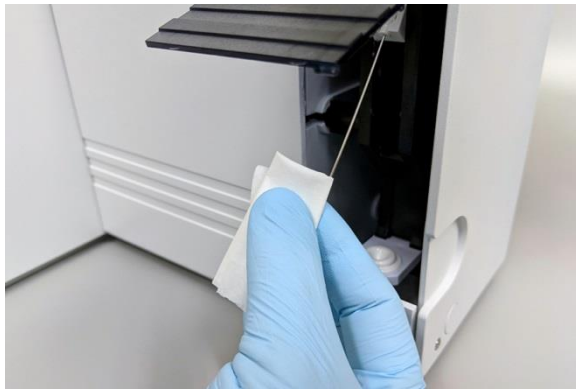
Figure 3-4 Wiping sample probe
