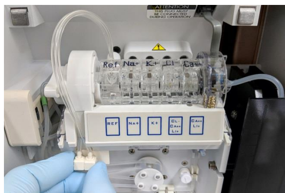
Figure 5-7 Plug in reference connector
