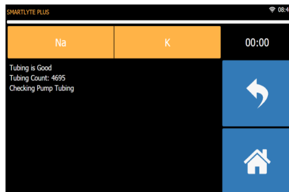
Figure 6-13 Pump tubing test in progress
