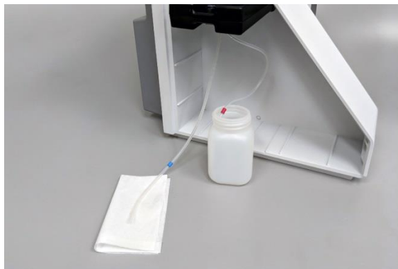
Figure 1-75 Water bottle removed
