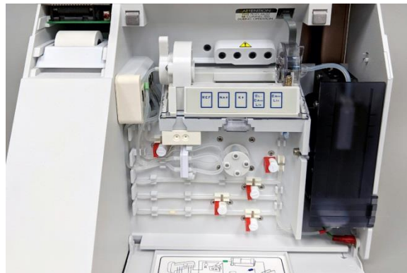
Figure 1-3 SMARTLYTE® PLUS with front cover open
