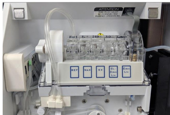
Figure 1-23 Electrode Tray in position
