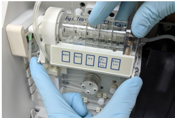
Figure 5-3 Pull electrode tray forward
