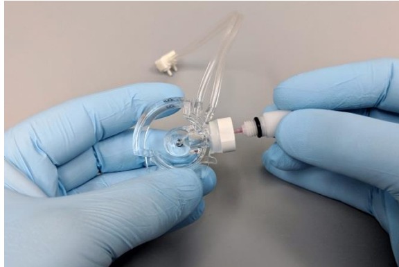
Figure 1-17 Electrode housing with Reference electrode
