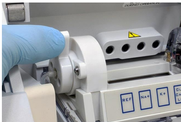
Figure 1-19 Unclamped electrode tray (unlocked position)
